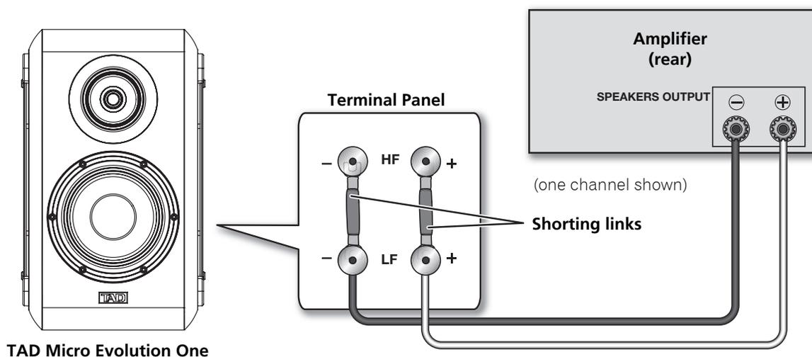
Figure 2. Connecting a speaker in a single-wired system
