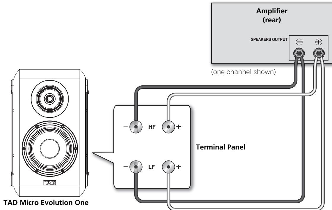
Figure 3. Connecting a speaker in a bi-wired system
