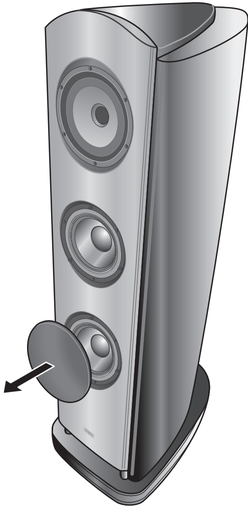
Figure 2. Removing the grille from the TAD Evolution One speaker system
