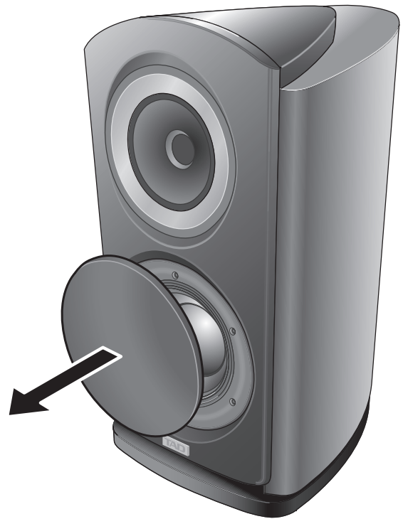
Figure 5. Removing the grille from the TAD Compact Reference speaker system
