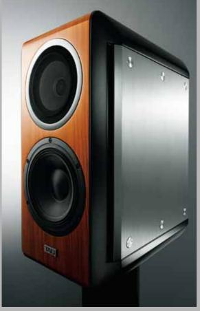
The SILENT\* enclosure brings together TAD's theory and technology. The cornerstones of its outstanding physical properties are its combination of birch plywood braces, MDF panels and Bi-Directional ADS Port featuring 10mm-thick hard anodized aluminum side panels that provide superior strength and vibratio dampening. Additionally, optimization of the enclosure Strong standing waves up to 250Hz.
